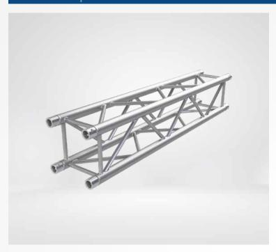
FD34 is the classic 29cm box truss that has proven itself over the years as the ultimate multipurpose truss. The straight elements lend themselves perfectly for spans up to 16m or as standard tower elements.
